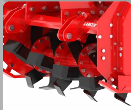
Helical Shape of Rotor Blades
