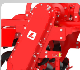
Heavy Chain Driven Side Transmission
