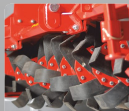
Helical Shape of Rotor Blades
